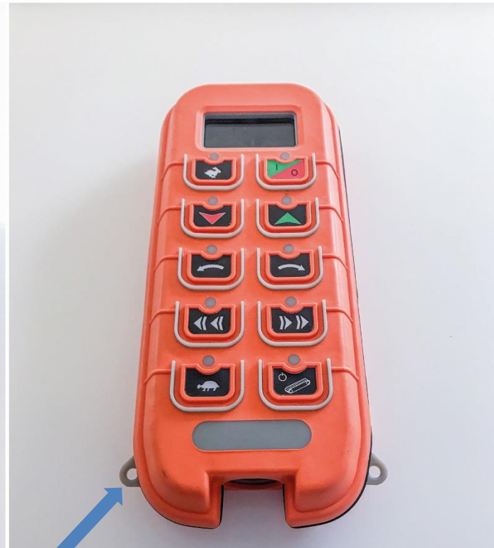
There were also fragile parts extending beyond the soft overmoulding which snapped under the drop test.
