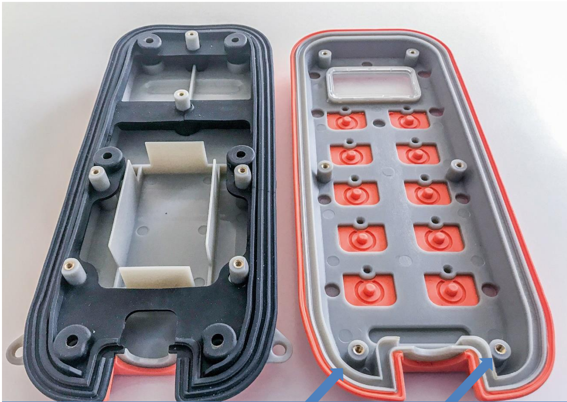
The fastening of the two halves of the electronics enclosure was placed inside of the seal so the device leaked when Ingress Protection tested.
