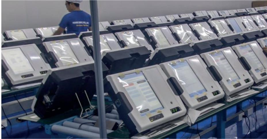
(Burn-in and testing of pilot production quantity)
