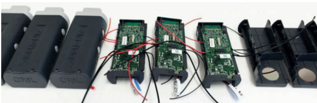
(Hand assembly of multiple units for clinical trials with production quality electronics)
