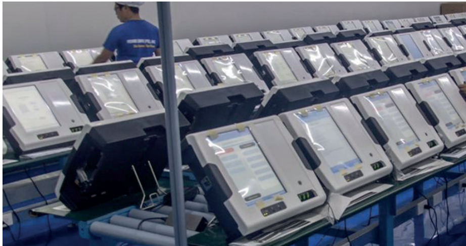
(Burn-in and testing of pilot production quantity)
