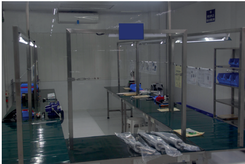
(Specialist clean room for small volume prototype medical device assembly)
